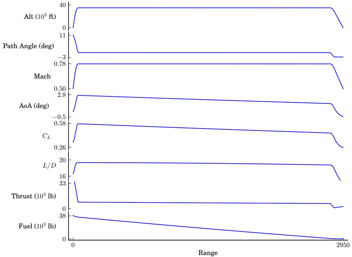
Figure 3: Boeing 737-800 mission analysis verification results.
