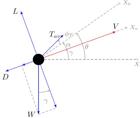
Figure 1: Free body diagram of flight equilibrium.
